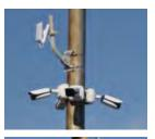
Pole-Mounted with 4 Pan-Tilt-Zoom (PTZ) cameras & loudspeaker
