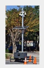
Free-Standing Pole with 4 Pan-Tilt-Zoom (PTZ) cameras & loudspeaker
